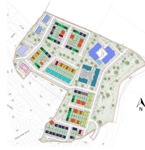
Proposed Site plan - Housing types
